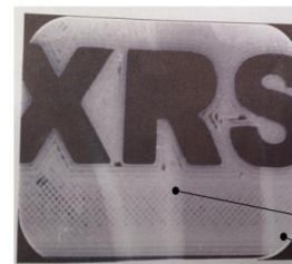
PLA based radio opaque XRS 80% infill / 5 mm thickness
